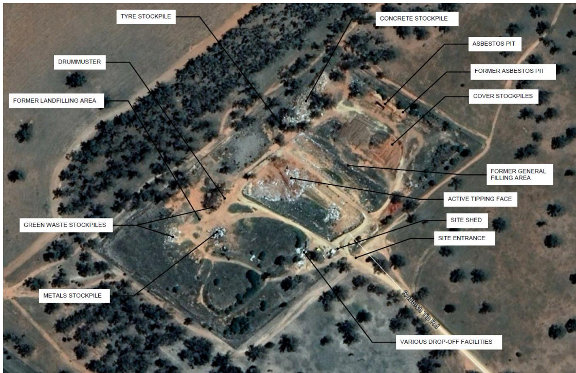
Figure 4.2 Trangie WMF existing site layout
